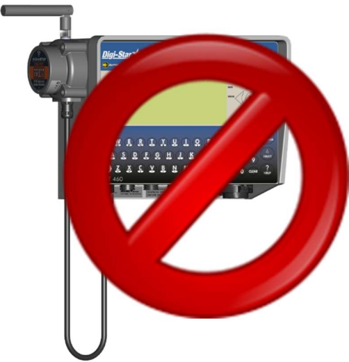
Figure 4. ERM-WiFi Incorrect Antenna Orientation
