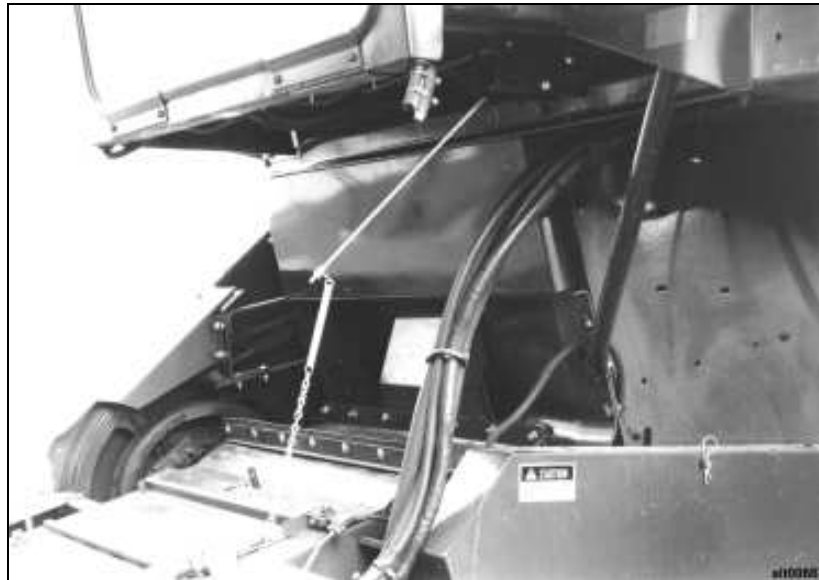
Figure 8. Header height sensor installed
