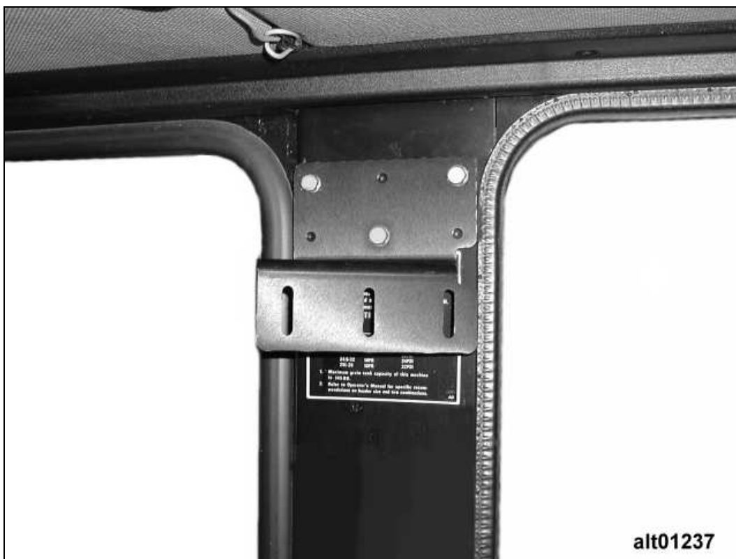
Figure 1. Post bracket installed
