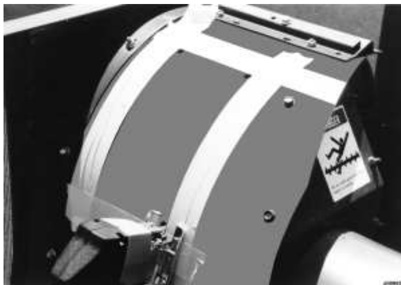
Figure 10. Section to be cut outlined with tape
