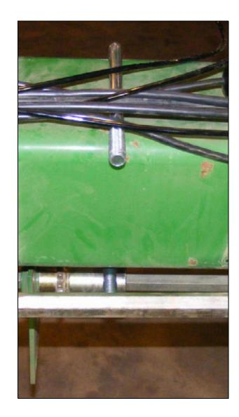
Place the mounting bracket on the implement and secure using the u-bolt and hardware provided.
