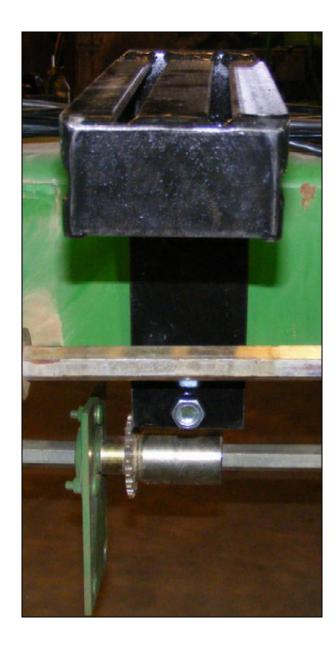
Place the variable rate drive on the mounting bracket and secure with the hardware provided.
