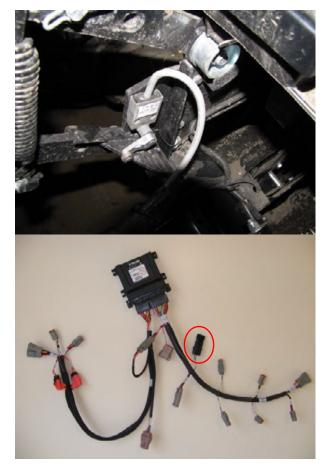
Use the appropriate adapter cable for your planter and implement switch to connect your specific switch to P5.
