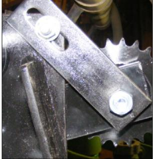
Install the double reduction gear.
