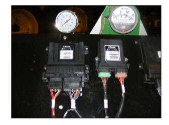
Connect the 18-pin Cinch connector on the CAN backbone adapter cable to the module.
