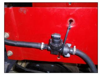
Attach the air line from the Tru Count control module into the LiquiBlock air hose adapter.
