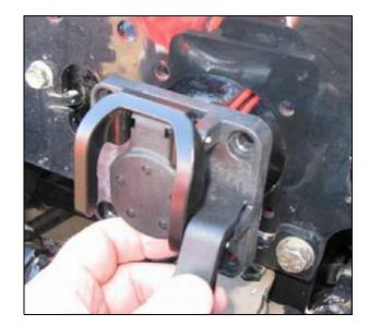
Connect the 4-pin DT plug (① shown in the picture) on the CAN cab harness to the 4-pin DT receptacle on the Powell connector (③ shown in the picture).
