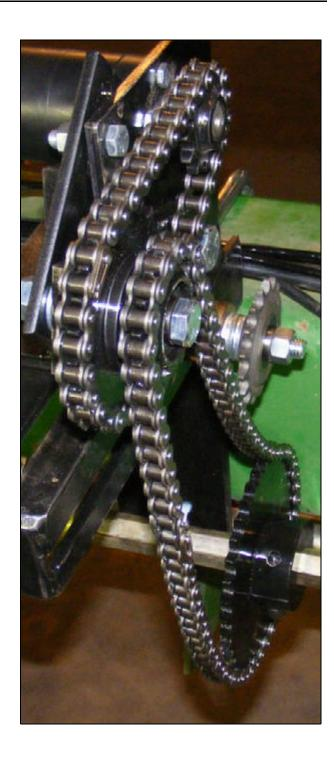
Tighten the idler sprocket.
