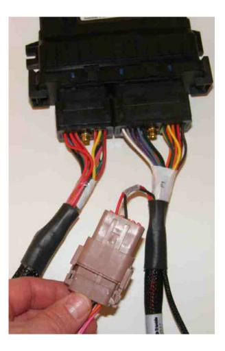
Connect the seed sensor harness to the adapter cable. See above for the correct style of adapter harness.
