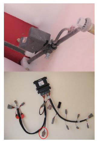
Use the appropriate adapter cable for your planter and bin level sensor to connect your specific bin level sensor to P4.
