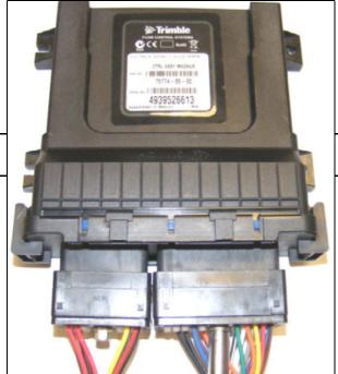
Connect the 4-pin DT and 4-pin DTP connectors to the CAN extension harness.
