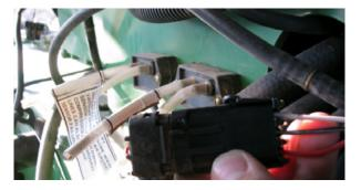
Use the appropriate adapter cable for your planter and pressure or vacuum sensor to connect it to P6 or P7 on 80540.
