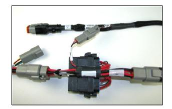
Connect the 2-pin connector on the relay to the 2-pin receptacle on the cab to hitch harness.
