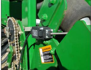
Connect the implement switch to the extension cable or to the control module. Route the cable to the control module and connect the extension cable to the module.
