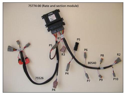
**Note** – Cables and connections are shown with the Rate and Section Control module. Cables 75526 and 80540 are also used for the Rate Control Only module and Section Control Only module when used with the FmX integrated display.
