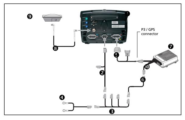
**CAUTION** – Connecting the Port Replicator on the CFX-750 display to NavController II cable to the P4 or P12 connector of the NavController II harness () will result in damage to the CFX-750 display and will void the warranty.
