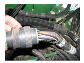
Connect R2 and P10 on cable 80540 to the appropriate row sequence on the clutch adapter harness.
