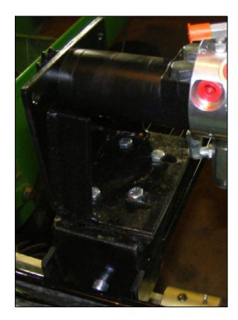
Install the double reduction gear mounting brace.
