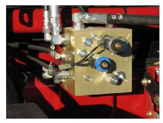
Use the appropriate adapter cable for your planter and valve type to connect your specific valve to P9.
