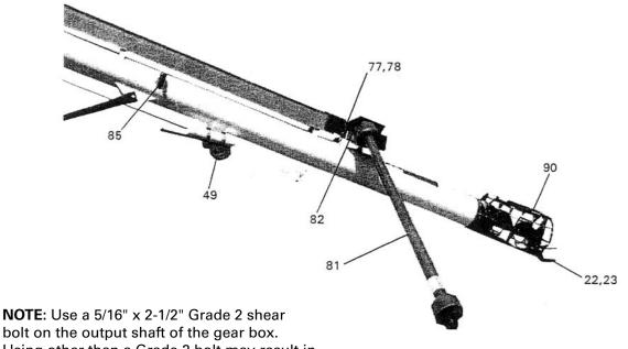
bolt on the output shaft of the gear box. Using other than a Grade 2 bolt may result in damage to the drive components.
