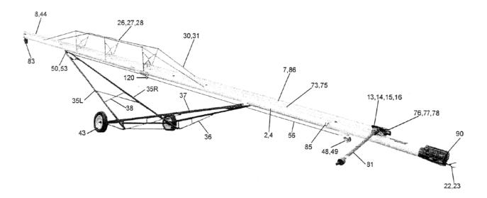
**NOTE**: Use a 5/16" x 2-1/2" Grade 2 shear bolt. Using other than a Grade 2 bolt may result in damage to the drive components.
