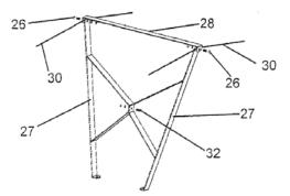
9. Mount the truss riser assemblies as instructed below.
