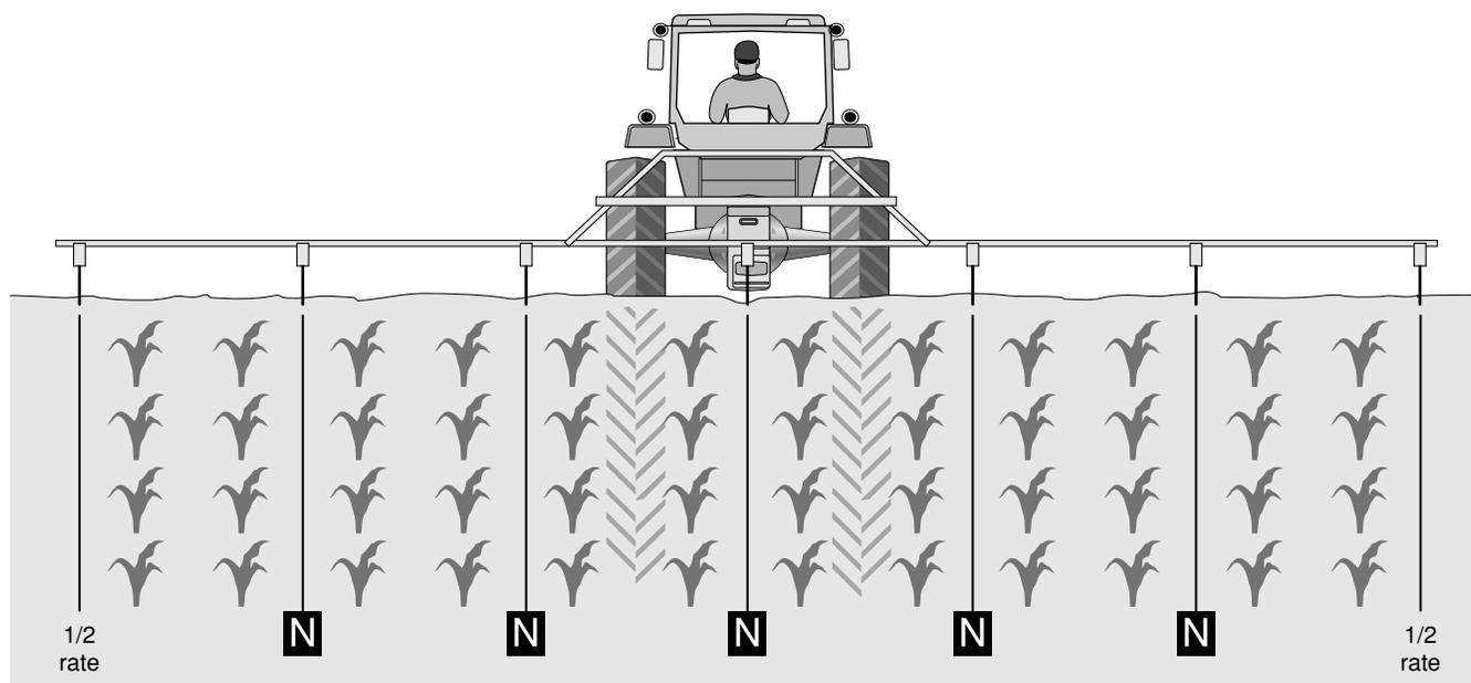
**Figure 11.10. Schematic of every-other-row, sidedress nitrogen injection. The outside two injectors are set at one-half rate because the injector runs between those two rows twice.**
