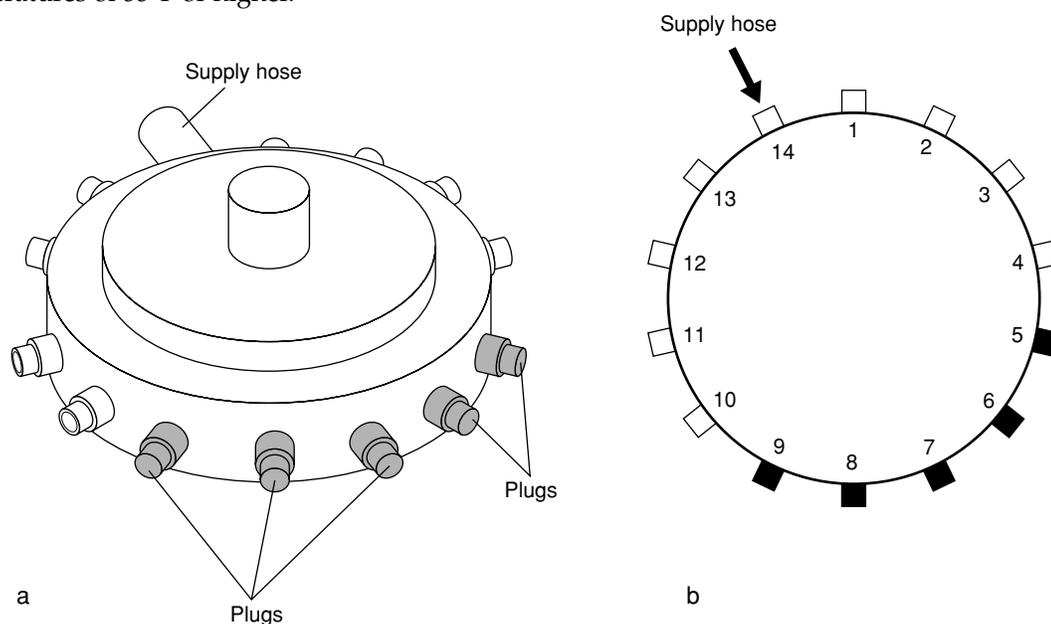
Figure 11.12. If plugs are needed on side-loading manifolds (see a), they should be placed directly across from the entry of the ammonia (see b).
