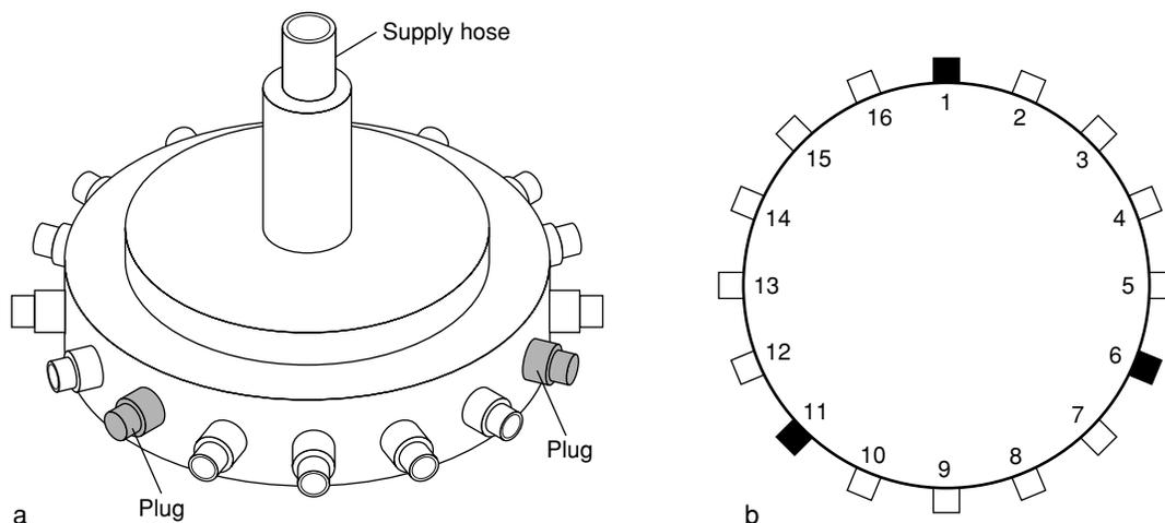
Figure 11.11. If plugs are needed on top-loading manifolds (see a), they should be placed uniformly around the manifold (see b).
