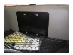
Step 2: Slide the NAV II box off of the threaded studs to expose the connectors on its right side. There is a 12-pin Deutsch plug labeled "Controller Diagnostics."
