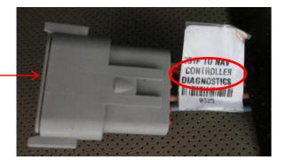
Step 3: Connect the 12-pin Deutch connector on the 727131 Trimble GPS Adapter to the 12-pin Deutch "Controller Diagnostics". Connect the 4-pin AMP "**GPS Port 1&2**" to the "**GPS**" port on the SeedSense tractor harness.
