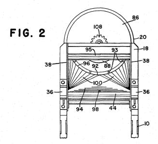
INVENTORS C. S. MORRISON H. H. DENISON THRESHING CYLINDER IN COMBINATION WITH A ROTARY SEPARATING DRUM
